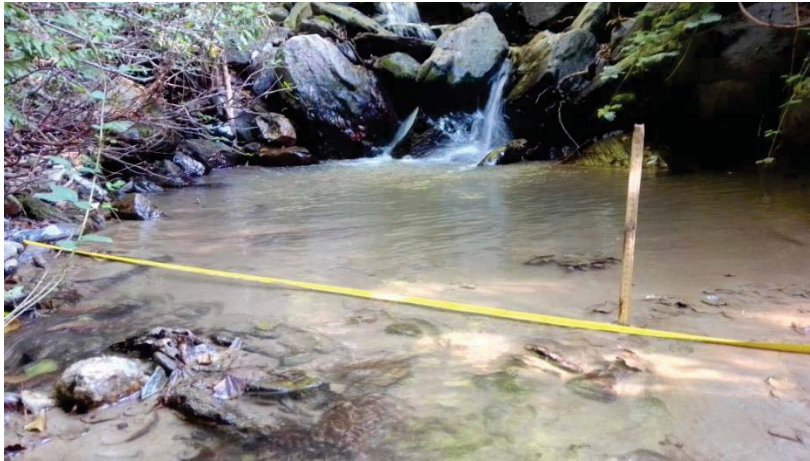
Fig 11: Transect where sediment thickness is measured in Pool 2.
