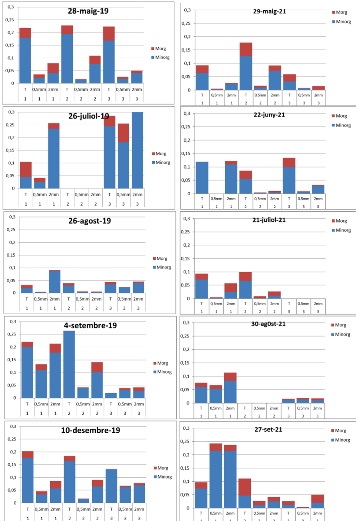
Fig. 9 Sediments transported -gr/day- in B6 of inorganic (blue) and organic matter (red), separated in 3 size classes: 2mm: greater than 2mm; 0.5mm: greater than 0.5mm and less than 2mm and T: less than 0.5mm; in localities: 1.- point above the track, 2.- point below the track, 3.- point downstream. Right column: pre-action samples, left column: post-action samples. The X indicates the lack of data due to the disappearance of the traps.
